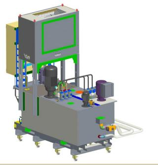
The image shows a complete IFDR 800/25 fine filtration system fitted with a delivery pump 20 bar 35 L/min and a delivery pump 70 bar managed by the inverter and the proportional valve, programmed to perform 6 pressure steps at these values: 20, 30, 40, 50, 60, 70 bar with maximum flow rate 45 L/min, and chiller for coolant's temperature control. This solution is dedicated to lathes with two spindles and 2/3 turrets, which need high and low pression on the tools.
