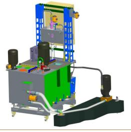
The image shows a complete IFDR 500/25 solution fitted with a delivery pump 20 bar 35 L/min and a delivery pump 70 bar managed by the inverter and the proportional valve, programmed to perform 6 pressure steps at these values: 20, 30, 40, 50, 60, 70 bar with maximum flow rate 40 L/min.
