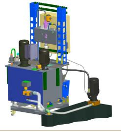
The image shows a complete IFDR 300/25 fine filtration system fitted with a delivery pump 20 bar 35 L/min and a delivery pump 70 bar managed by the inverter and the proportional valve, programmed to perform 6 pressure steps at these values: 20, 30, 40, 50, 60, 70 bar with maximum flow rate 40 L/min.
