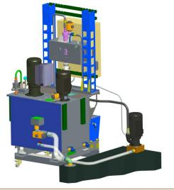
The image shows a complete IFDR 300/20 fine filtration system fitted with a delivery pump 20 bar 35 L/min and a delivery pump 70 bar managed by the inverter and the proportional valve, programmed to perform 6 pressure steps at these values: 20, 30, 40, 50, 60, 70 bar with maximum flow rate 33 L/min.
