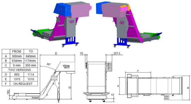
The dimensions A, B, and C can assume the following values (mm) to adapt the conveyor to the tank of the machine tool.
