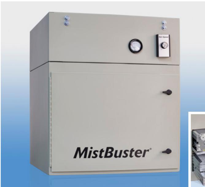
A media-based air filtration system for the collection and removal of mist, smoke and metal particles produced by machine tool operations. The system uses 58 sq. ft. of lofted micro-fine fiberglass media in its second filtration stage.
